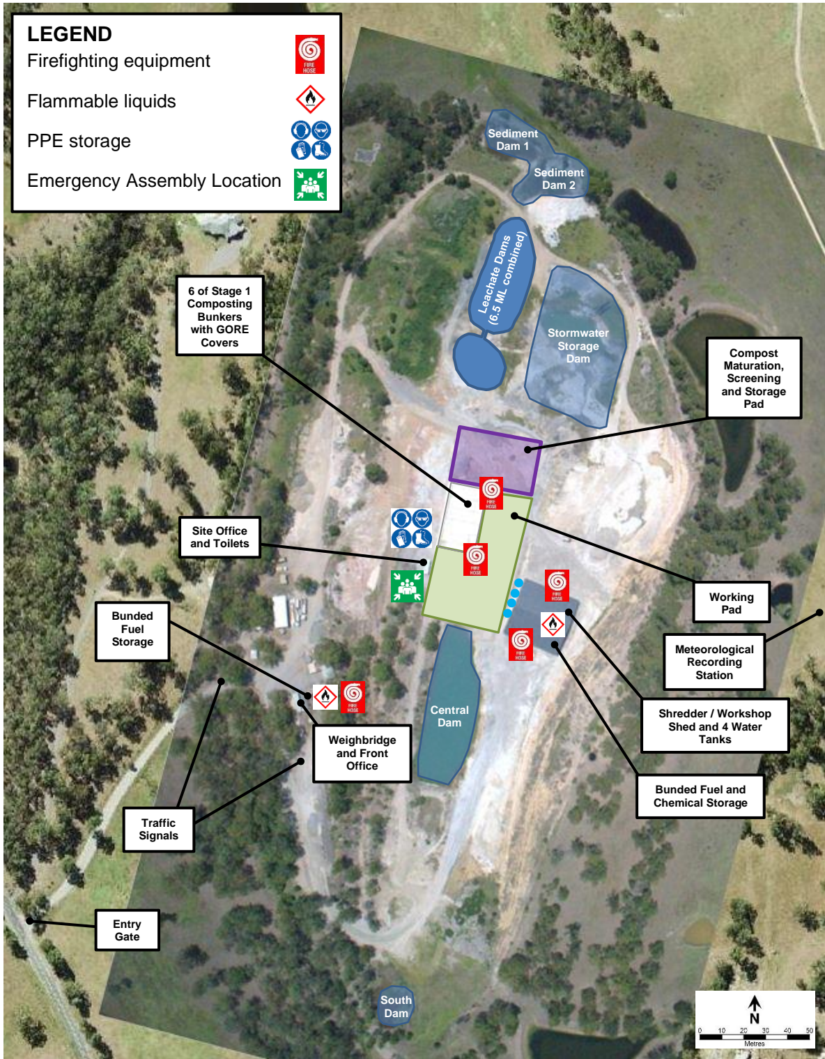
Figure 4 – Site locations of flammable liquids storage, firefighting components, PPE storage and emergency assembly point
